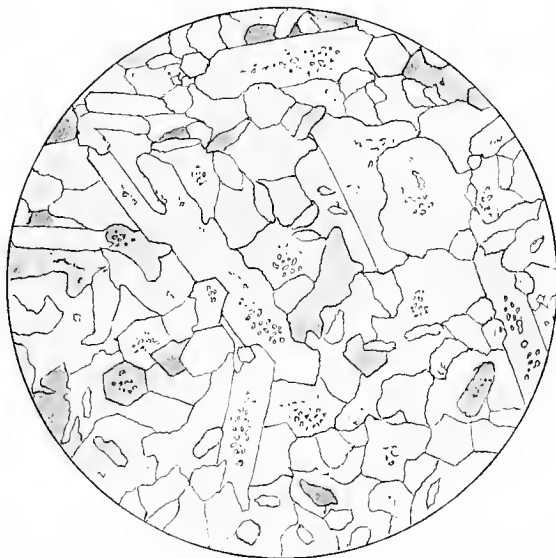
Silicified Limestone ("Jasperoid"). Aspen, Colo. Crossed nicols. All quartz. Small inclusions of calcite in some of the grains. Magnified 30 diameters.
